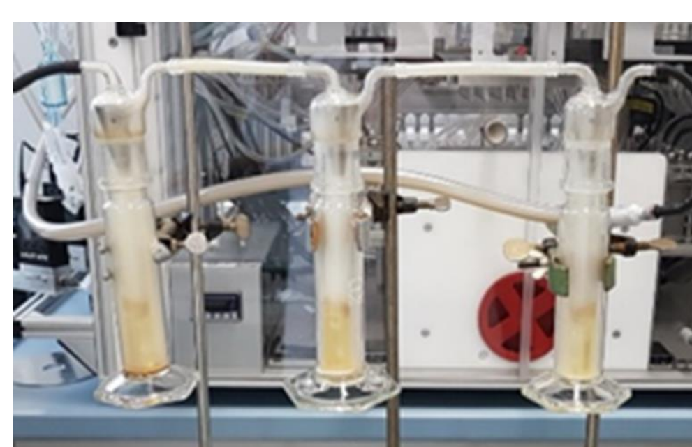
Figure 1: Bubbling smoke/aerosol exposure system
